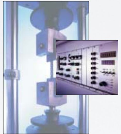
For the testing of fatigue strength, we use, among others, this – designed according to the latest technological knowledge – high frequency fatigue testing machine.
