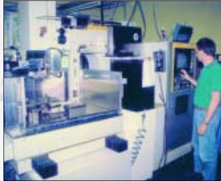
This jig boring machine plays a large role in the precision of the Rexnord chain tools.
